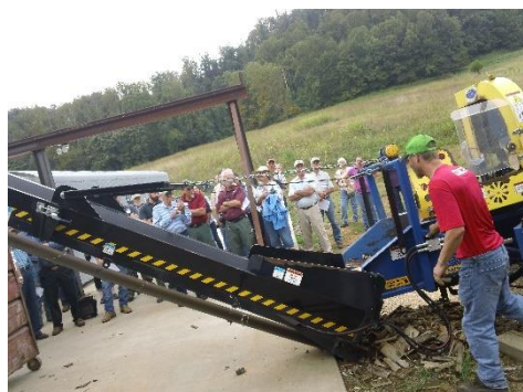
Jason Drew, Cahas Mountain Charcoal employee, demonstrates wood block cutting then transporting via conveyor system to storage bin before placing in drying oven.
